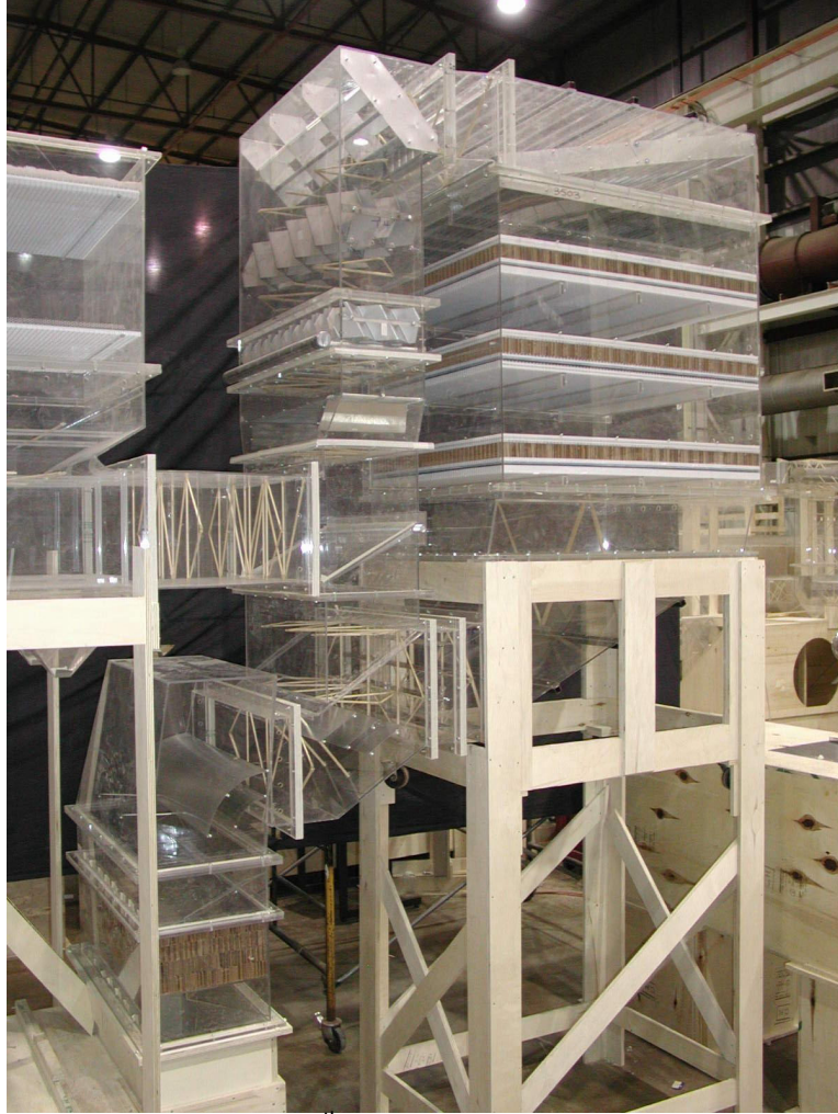
Figure 5 - 1/12 th Scale Flow Model (Unit 3)
