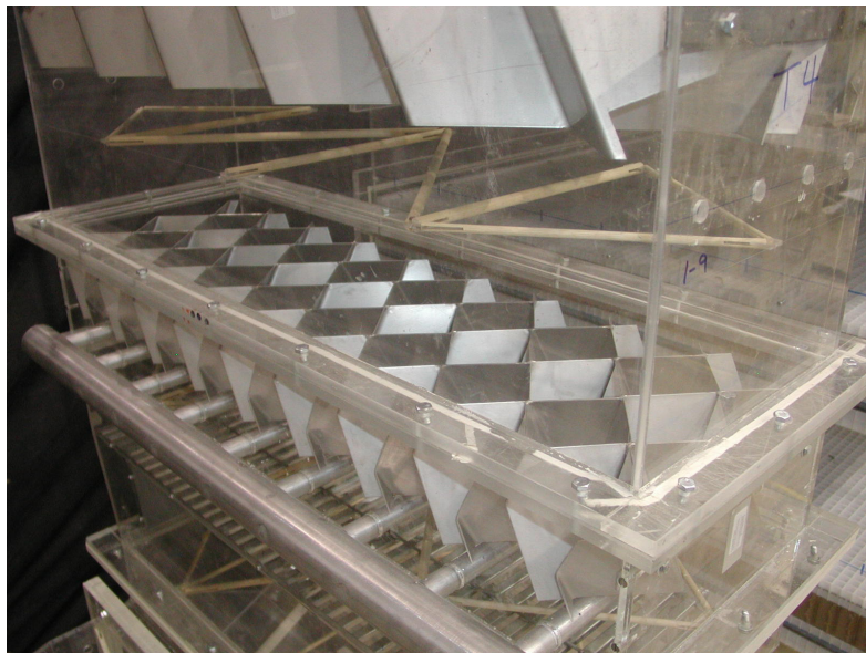
Figure 6 – Scale Model of ALG and Static Mixers (Unit 3)
