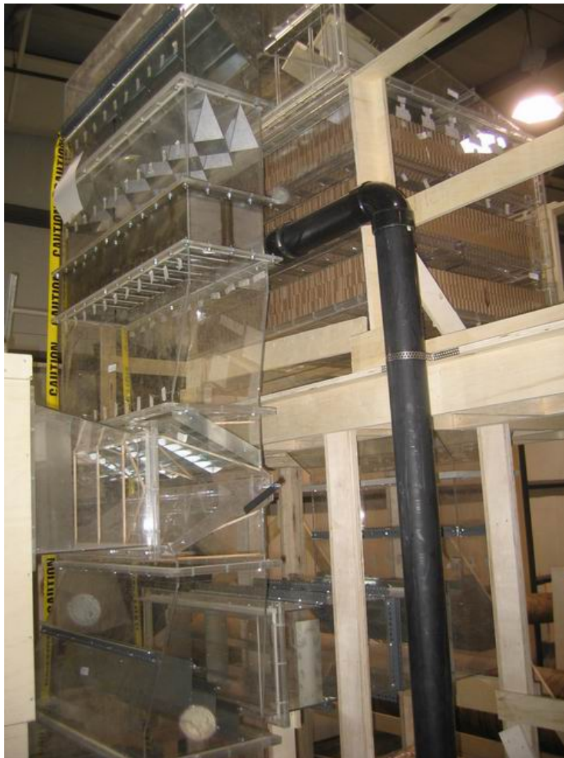
Figure 7 – 1/12 th Scale Physical Flow Model
