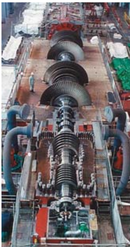
Steam turbine for Hokkaido Electric Power Co., Inc., Japan Tomato-Atsuma Power Station No. 4 700MW, TC4F-43, 3,000 rpm, 25.0 MPa, 600/600°C Put into service: 2002
