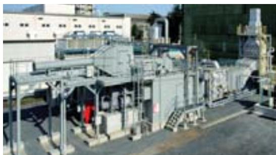
AHAT(Advanced Humid Air Turbine) System pilot plant at the Katsuta Research Center.
